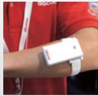
**NTT Docomo** displays devices that measure acetone emitted from the skin, providing a visual representation of fat burning
